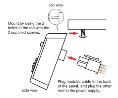
**NOTE:** Connect only the RED and BLACK wires to the power supply wiring harness.
